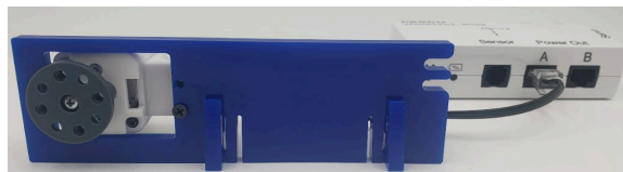
Figure 1. Stepper Attached to Bracket
