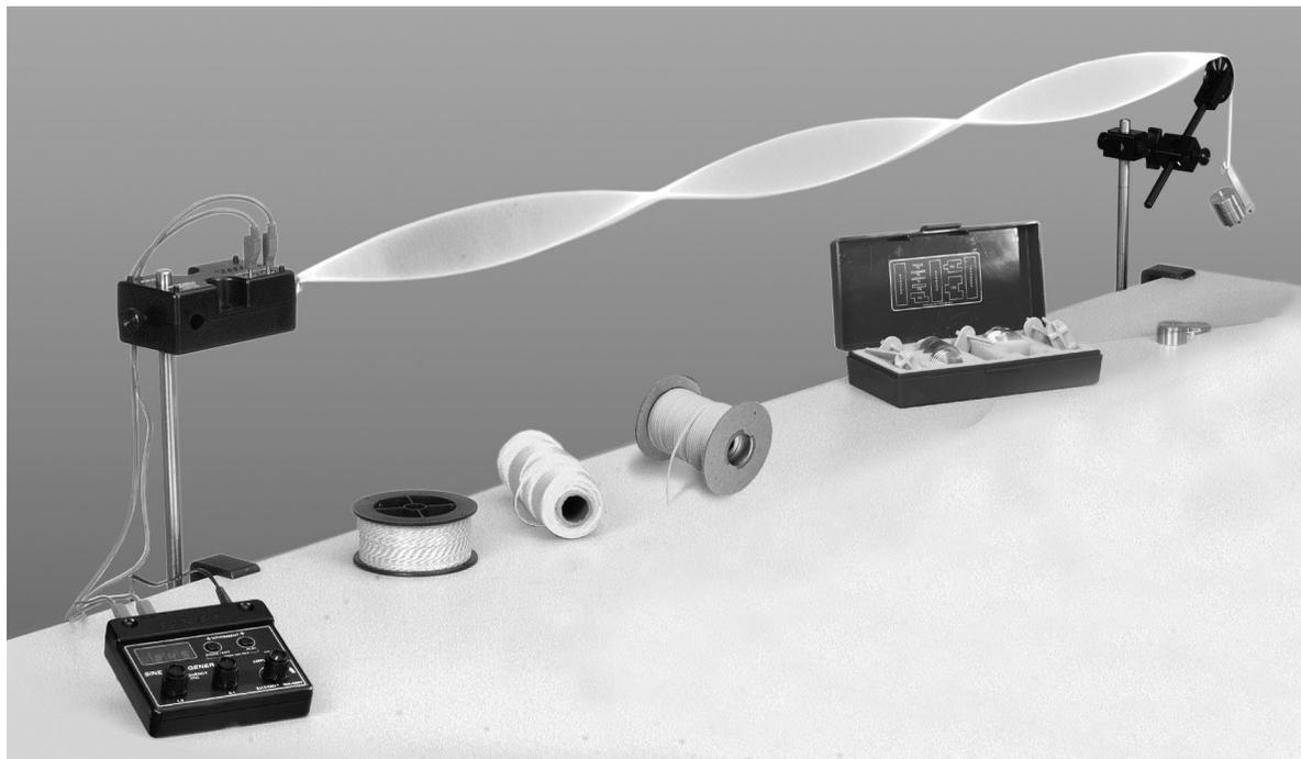
3. Measure from the knot where the string attaches to the string vibrator to the top of the pulley. This is distance  $L$ . (Note that  $L$  is *not* the total length of the string, only the part that is vibrating.)
