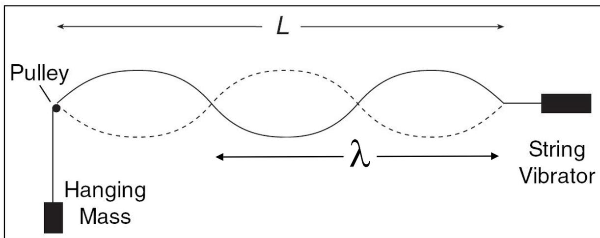
$L$  is the length of the vibrating part of the string and  $\lambda$  is the wavelength of the wave. For the string shown above vibrating in 3 segments,  $\lambda = \frac{2}{3} L$ .
