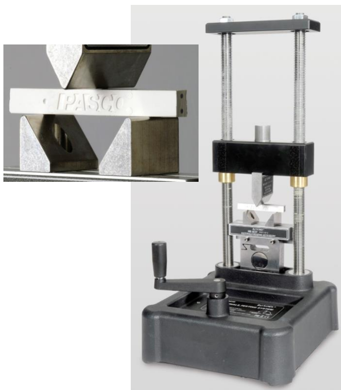
Figure 1: Three-point Bend Test
